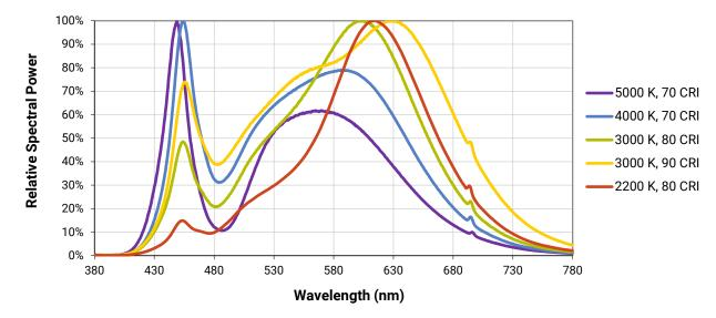
The following graph is the result of a series of pulsed measurements at 1900 mA and  $T_J$  = 85 °C.
