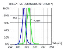
FIG.4 RELATIVE LUMINOUS INTENSITY VS. WAVELENGTH.
