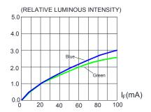
FIG.2 RELATIVE LUMINOUS INTENSITY VS. FORWARD CURRENT
