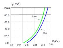
FIG.1 FORWARD CURRENT VS. FORWARD VOLTAGE.
