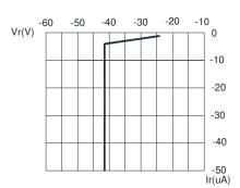
FIG.3 REVERSE CURRENT VS. REVERSE VOLTAGE.
