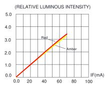
FIG.2 RELATIVE LUMINOUS INTENSITY VS. FORWARD CURRENT
