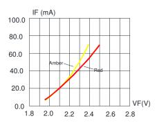
FIG.1 FORWARD CURRENT VS. FORWARD VOLTAGE.
