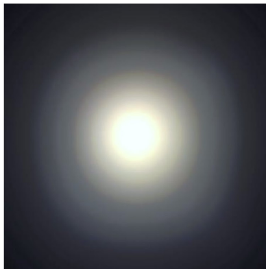
Figure 6: Luminance and color over angle data (top) with corresponding true color beam projection images (bottom) from the LEDiL CA11264 HEIDI-D optic
