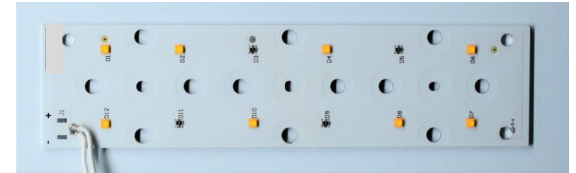
XP-G3 8-LED PCB used in this LED-based fixture retrofit
